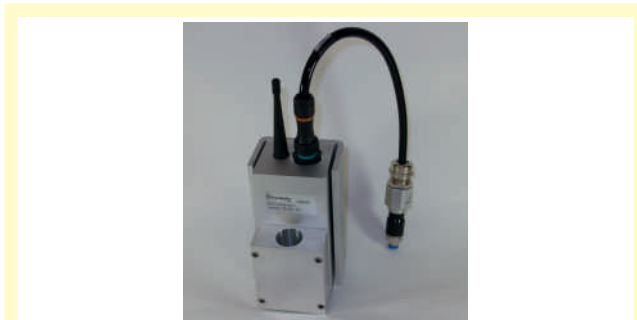
Figure 12: Realized sensor module with pressure and temperature sensor plug (Source: Fraunhofer IMS)
