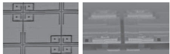
Figure 1: SEM image of a microbolometer (top view and cross section)
