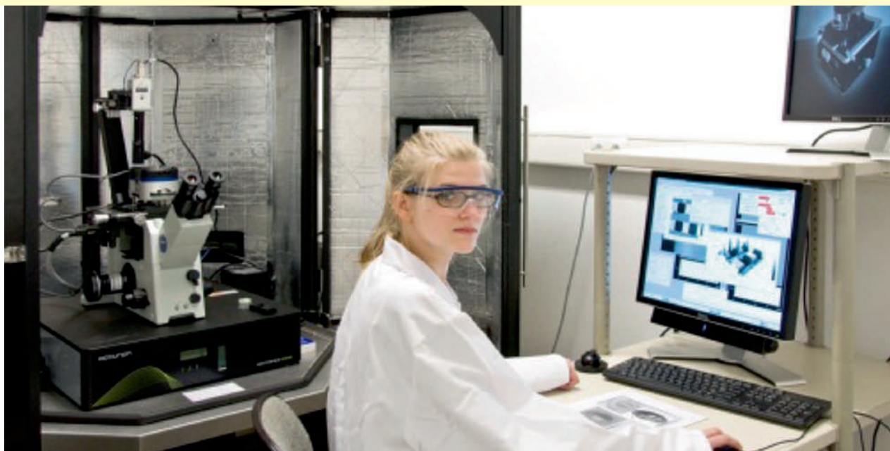
Figure 1: Quality control of an electrode-surface functionalized with the enzyme glucose-oxidase. The modern AFM (atomic force microscopy) in the Biosensor-Lab of FhG IMS is dedicated for measurements in liquids and biological samples in the (sub-)nanometer range.
