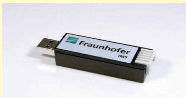
Figure 2: USB-stick potentiostat together with a software package brings electrochemical measurements as a plug-and-play solution to our customer.
